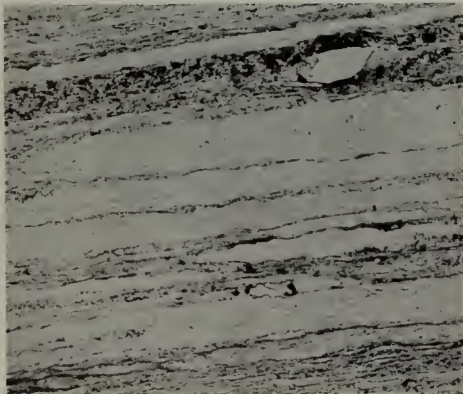
FIGURE 15. Photomicrograph of stretched conglomerate (X25). Section is taken normal to the shear cleavage and intermediate axes, showing long and short axes of stretched pebbles. Rock is composed largely of quartz and muscovite, with minor chlorite, albite and iron oxides. This rock has been considerably sheared and recrystallized and probably could also be called a phyllonite.
